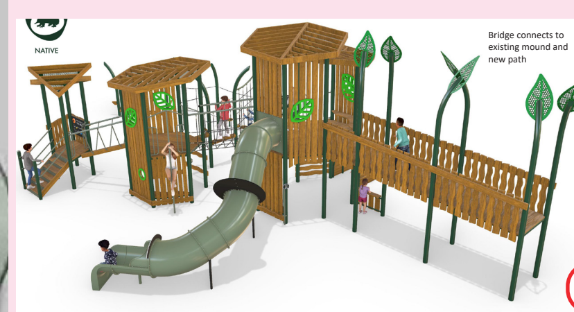
MULTI-ACTIVITY TIMBER and STEEL STRUCTURE with a variety of climbing activities, tunnel slide, fireman's pole, climbing nets, balancing, accessible upper deck and ground level cubby-house activities.
